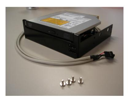
Put the drive bay assembly into the 5.25" bay on the back side of the robot. Using the bay shown has been found to be the best (in terms of cable lengths/ease of access) but any free bay can be used.
