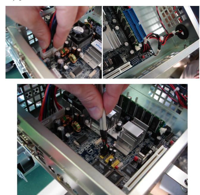
Plug in the USB connector running from the M3 motor and I/O controller into the back panel USB port of the Mini-ITX.
