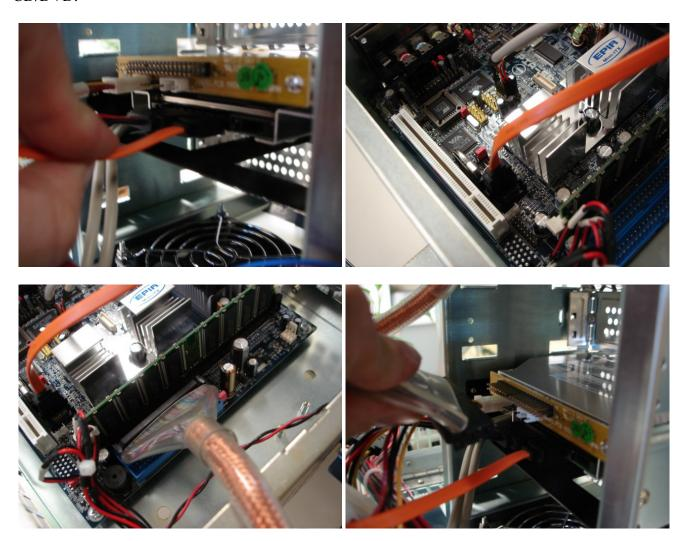
Verify the routing of cables for cleanliness and ease of closing side bays. It is also up to the customer to verify that the cables are not blocking the operation of any cooling fans on the Mini-ITX.
