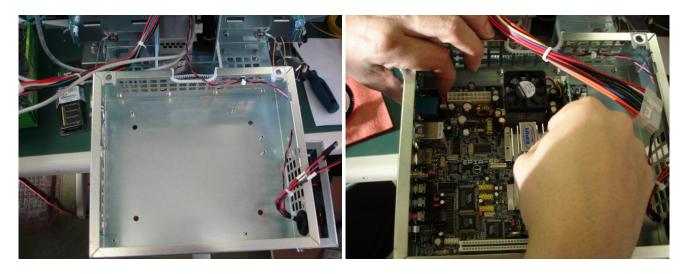
**Step 17**Screw down the Mini-ITX board with the four M3 screws.
