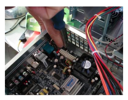
Using the user manual and/or datasheets as guides for your Mini-ITX, plug in the various connectors to the board. For the recommended VIA SP13000 Mini-ITX, I start with the 20 pin ATX connector and then plug in the LEDs, ON/OFF/Reset switch and USB header connectors.
