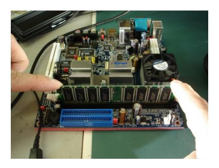
Move the harness out of the way in the computer side bay and place the Mini-ITX down over the stand-offs and into the back-panel plate. The screws for mounting should already be in the stand-offs and will need to be taken out before doing so.
