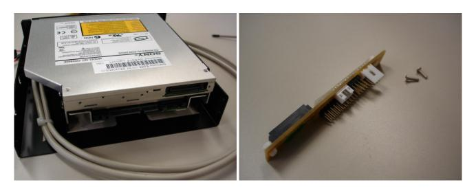
Push the adapter board onto the back of the Slim CD/DVD drive connector and use the screws to hold it in place firmly.
