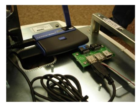
In this location the head can still be placed back on the robot and not interfere with the Wireless USB Network Adapter or its antennae.
