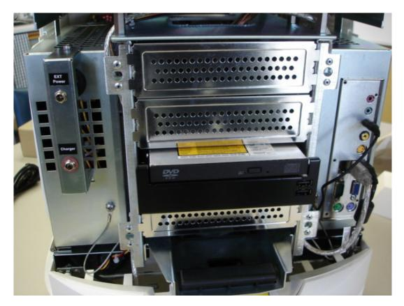
Plug the monitor, keyboard and mouse into the Mini-ITX back panel in order to setup Windows. You will also need an Ethernet connection to be able to register Windows.
