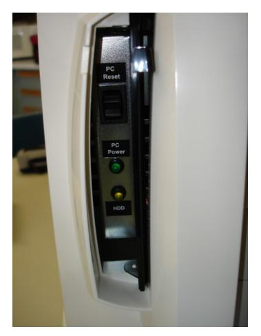
As with other PCs, you may control the behaviour of the "PC Power" button from the Windows Control Panel. It is recommended to configure the power button to 'Shutdown', your robot's PC should already be set in this way when you receive it.
