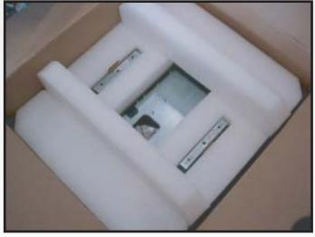
To remove the robot from the box you will first need to remove the top protective foam as shown in the following picture. Gently grab the foam piece from the fins on top and pull straight upwards.
