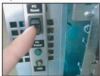
Finally, the switch for PC Power is still available and can still be used by the User by pushing down on the toggle switch. The PC Reset is the same switch, only pushed upwards.
