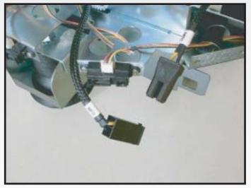
BEFORE you can turn on the robot you must connect the batteries to the power supplies.
