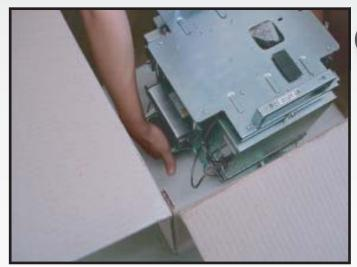
Reach into the box and lift the robot out by the handles.
