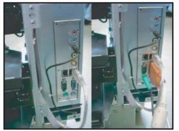
Once the plug is connected, connect your monitor, keyboard and mouse to the back of the Mini-ITX computer located in one of the fold down bays.
