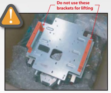
The handles are NOT the metal brackets visible on the top of the robot in the above diagram. The proper handles are located lower on the robot's body at the bottom of the drive bays.
