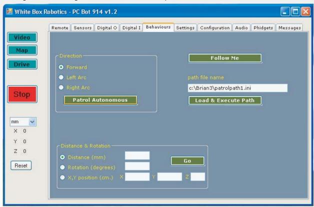
You will need to keep an eye on your robot and be ready to press the red "Stop" button until you have properly configured your robot's IR sensors, speed, velocity, acceleration, etc. to your robot's environment. You may even change the positions of the 8 IR sensors that are provided. Consult the BRIAN Developer's Guide for details, and please see our forums at:
