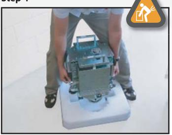
Place the robot down on the ground, with the foam still attached. Either hold the foam with your feet or have someone hold the foam while you pull the robot free.
