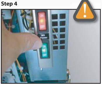
Next turn on the M3 Controller power. If this switch is OFF the M3 will not be able to drive the motors or read the sensors.
