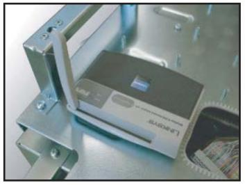
Once attached rotate the antenna to the upright position.
