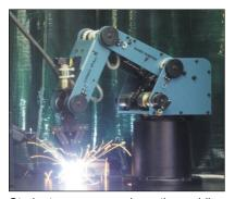
Students program and practice welding techniques in simulation and then execute automated welding applications online using the automated welding workcell.
