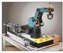
Students learn to program and operate the SCORBOT-ER 4u and auxiliary servo and I/O devices using both actual and simulated robotics and materials handling workcells.
