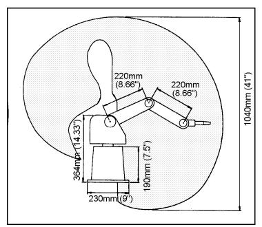
Figure 6: Operating Range (Side View)
