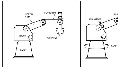
Figure 2-3: Robot Arm Links
