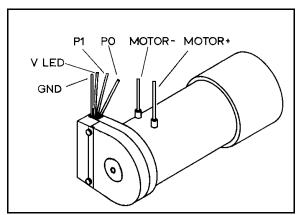
Figure 25: Motor Wiring
