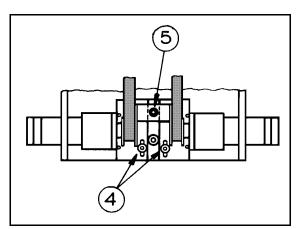
Figure 18: Tightening Belts in Robot Base
