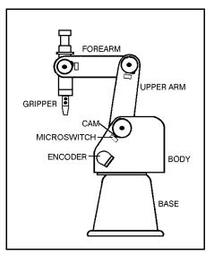
Figure 2: Robot Arm Parts
