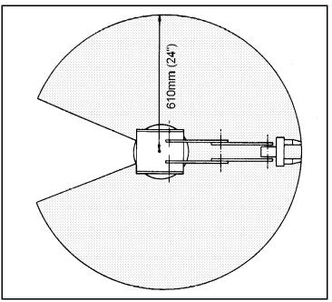
Figure 5: Operating Range (Top View)
