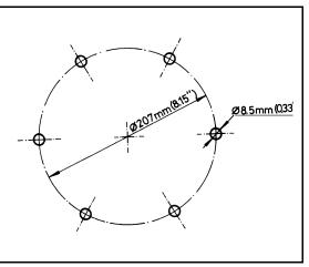
Figure 13: Robot Base Plate Layout
