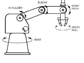
Figure 2-4: Robot Arm Joints
