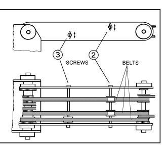
Figure 17: Tightening Belts in Upper Arm
