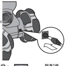
**NOTE:** Mr. Personality will only bend at the waist, perform arm movements, and media functions (that is, he will not perform any movements on his wheels) when being powered by an adapter.
