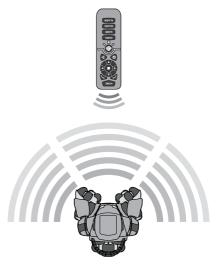
**NOTE:** Avoid using the Homing function in a cluttered area, as it will confuse Tri-bot and make it harder for him to detect the homing signal. Tri-bot's IR sensors are based reflection. He can see highly reflective surfaces, such as white walls or mirrors more easily and from greater distances than matte or black surfaces.
