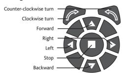
To control his movements you can use the direction pad on the remote controller. For example, press the left direction button, to move Tri-bot to his left. To make him turn on the spot, use the arrow buttons for either clockwise, or counter-clockwise turns.
