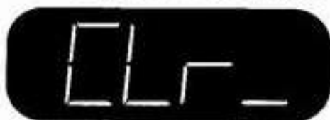
CLEARING PROGRAM STEP
