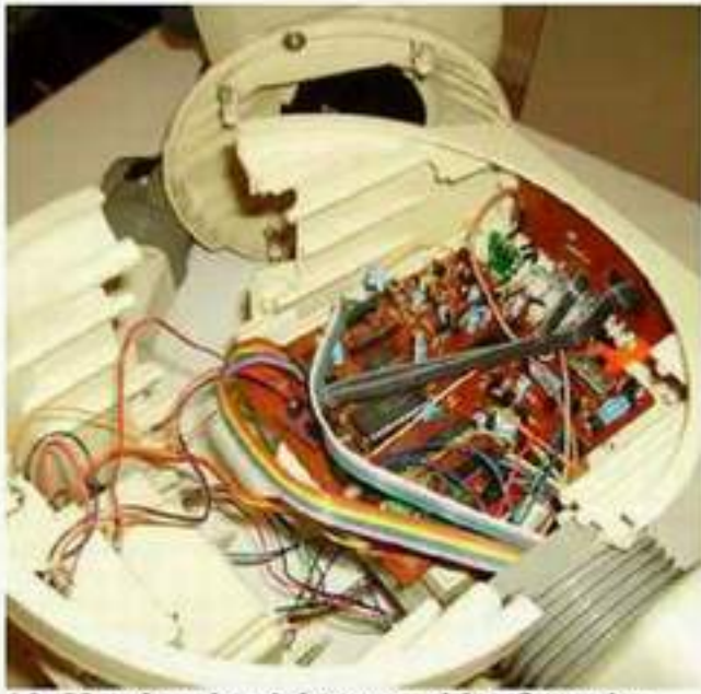
12. Un-plug the right arm cables from the circuit board, two cables and plugs.
