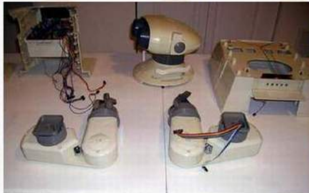
17. You have now disassembled the major components of the robot. Disassembly of the components will be addressed separately. To reassemble the robot reverse the procedure.
