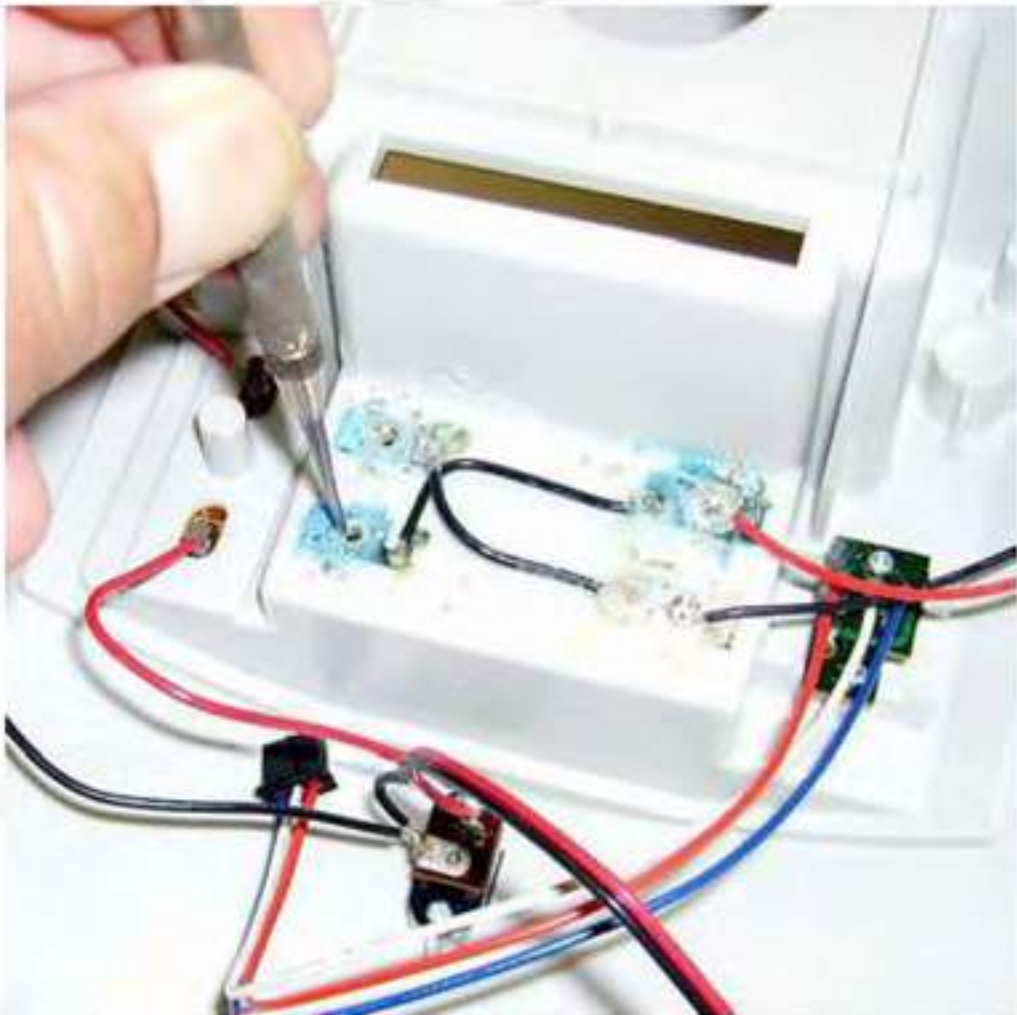
5. Once the eye lit ridge is removed take a punch smaller than the hole and gently tap all four of the eye lit out.
