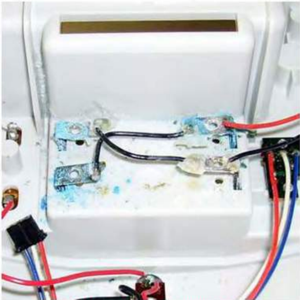
7. Gently pry the battery contacts out.
