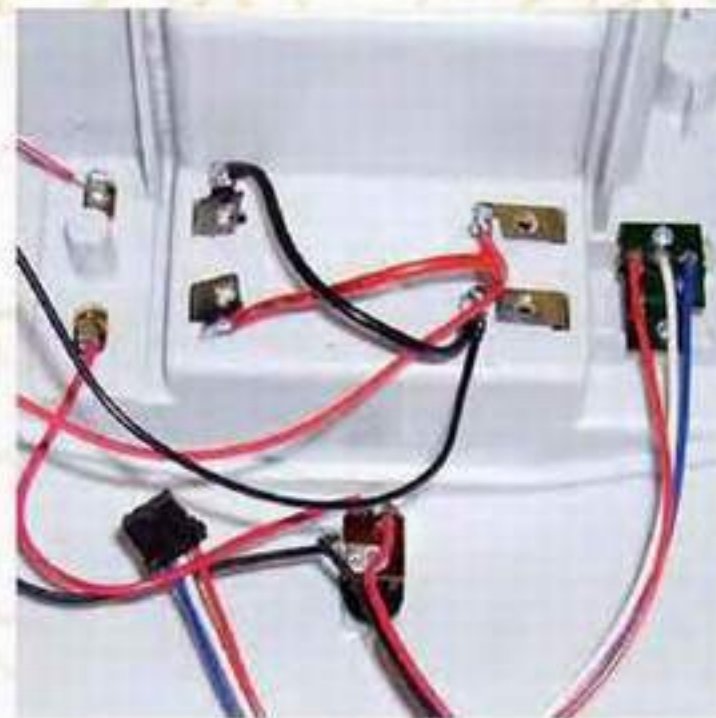
10. After cleaning the housing reinsert the new battery contacts and wires in the housing.
