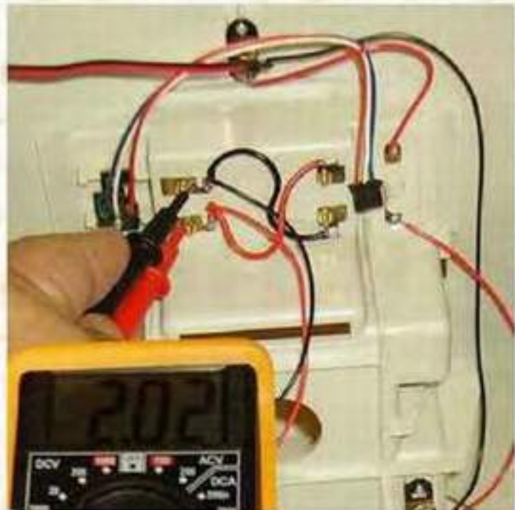
15. Use a multi-meter to check conductivity both at the rear and the plug. The operation is finished.
