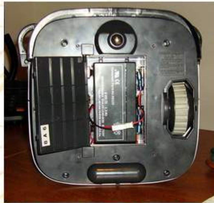
5. Plug in the battery and close the door. (You are ready to go.) Click to Enlarge
