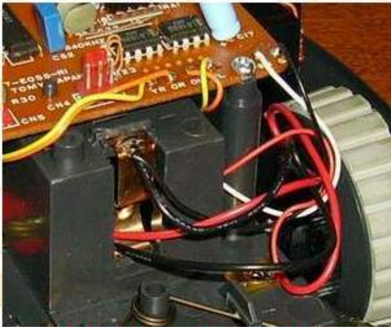
4. Solder the plug and wire to the (+) positive and (-) negative terminals as shown. 5. Reassemble the robot. Click to Enlarge
