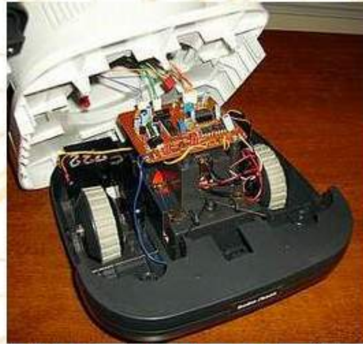
2. Turn the robot up and separate cheerfully. 3. Unplug the five plugs from the robot. (They are keyed and color and pin coded.) Click to Enlarge
