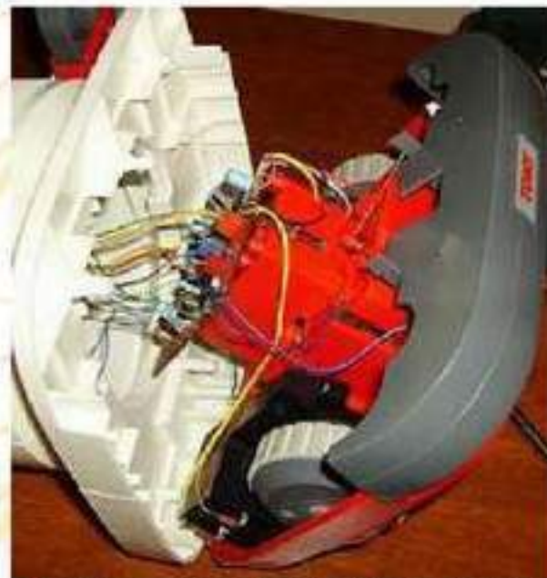
2. Turn the robot up and separate cheerfully. 3. Unplug the five plugs from the robot. ( They are keyed and color and pin coded. ) Click to Enlarge
