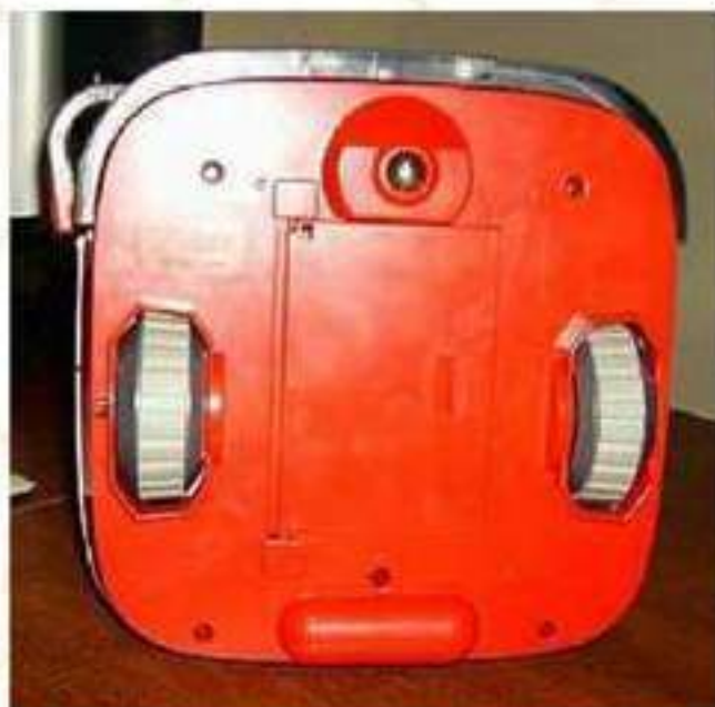
1. Take five screws from the bottom of the robot.
