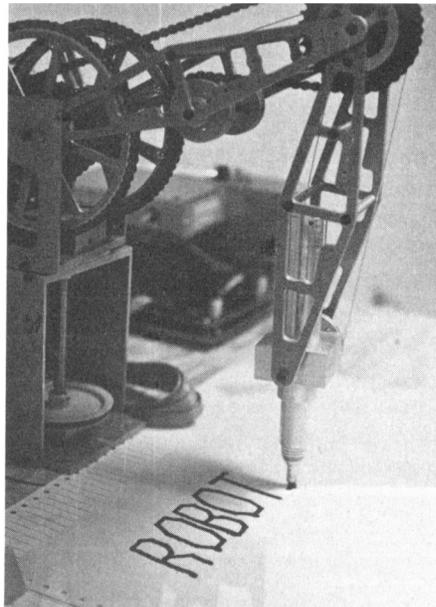
from 0 to 121, since the feedback registers on the Rhino's Intel 8748 control processor use the high-order bit as a direction flag. Step commands larger than 127 drive the motors in the reverse direction intended, for the number of steps in excess of 127.
